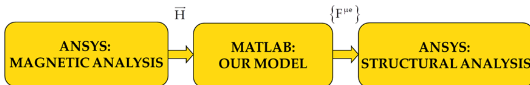
Figure 6. Forward coupling used to compute the magnetostriction strain of the test bench.
