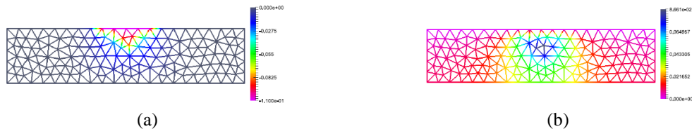
Fig. 13 Coupled soil-foundation system (a) vertical displacements (b) excess pore pressures ( k=1 \cdot 10^{-6} m/s, \nu=2 \cdot 10^{-5} m/s)
