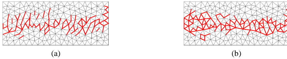
Fig. 5 Elements with increasing damage (a) mode I (b) mode II (note that we mark the cohesive links that are activated by cracks)
