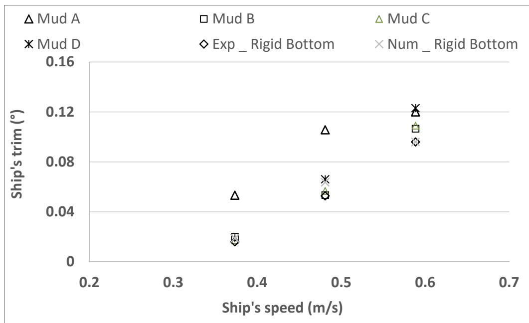
579 580 Figure 25. Ship trim as a function of the mud properties for an UKC of +10%.
