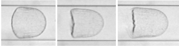
Figure 1: Pictures of ovalbumin microcapsules flowing in a microfluidic channel (cf Chu et al. (2011)).
