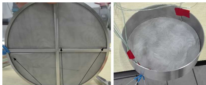
Tips of thermocouples
