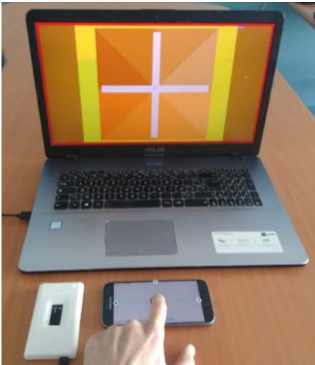
Figure 6 : The Tactos system equipment for the sessions (computer, MIT5 and smartphone)
