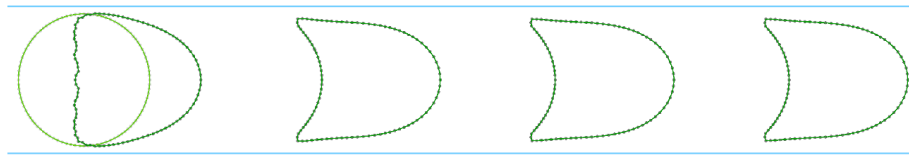
Figure 6. Sequence of cross-section capsule shapes and positions in the microchannel from the initial spherical shape shown in light green at the beginning of the channel: comparison of the FOM solutions (grey dots) and of the solutions computed from the dynamical k -DMD reduced-order model (dark green solid line) at the same instants as in Figure 1: t = 0, 0.4, 2.8, 5.2, 7.6 .
