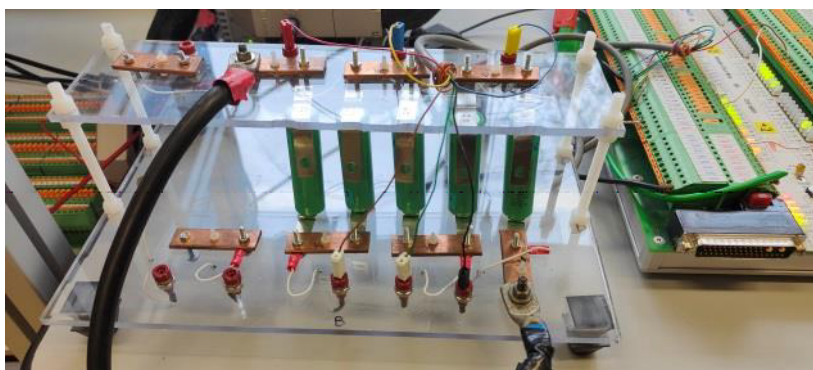
Figure 3: Battery pack made of 5 cells in series.
